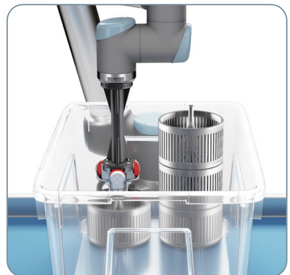
An EMI-designed plate EOAT removes the part from the mold and delivers it to the Cobot EOAT to be packaged.
