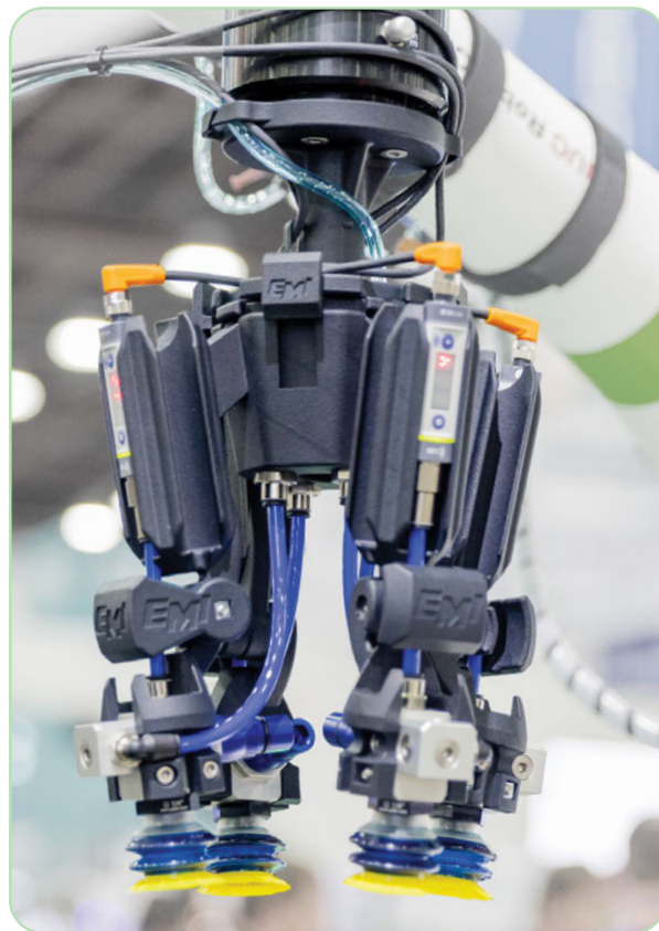
The electronic switches have a modular structure and can be easily integrated into the automation environment.
