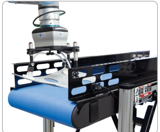
Above, EMI's End-of-Arm Tool removes the part from the injection mold, hands it off to the Cobot end effector customized by our Engineers, and delivers the workpiece to a Cobot-Ready Conveyor. EMI helped automate this real world application in a customer facility.
