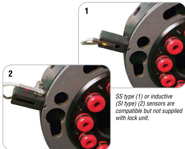
Electrical safety: It emits an electric signal, only when locked. This signal will give the consent to the movement of the robot. In the case of incorrect engagement, or destructive impact on the LOQC, or electrical fault of the sensor, the signal drops out and the robot stops.
