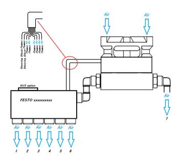
If in need of extra supply of air pressure, the second air port on the Tool Holder (TH) can be added on to the steering Block. (Picture example: Pneumatic steering Block FESTO VTUG-10-MSDR-B1TZ-25V20-Q10L-UL-Q6S-6P)
