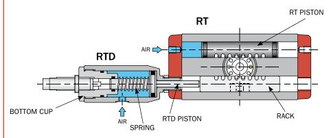
The RTD stroke can be easily adjusted by means of spacers to be placed in front of the piston, so that the intermediate stop can take place in different positions.
