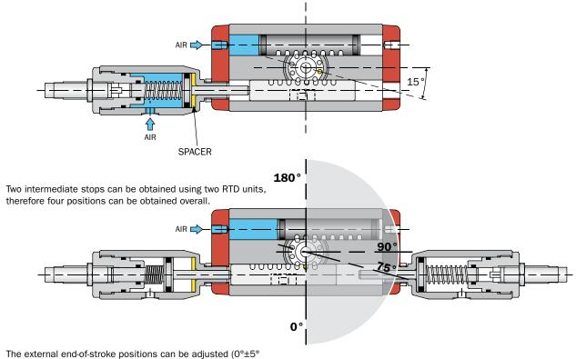
or 180°±5°) by means of the same devices as used in the RT (shock absorbers, rubber bumpers, stop dowels). The mid-stop position can be adjusted (90°±5°) by screwing/unscrewing the RTD in the RT.
