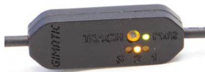
Output 2 - Gripper Mid-Stroke: (Part Gripped)
