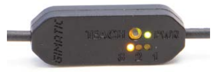
Output 3 - Gripper Closed: (Part Missed)
