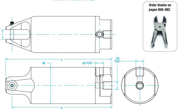
Note: Rotating endcap can change the orientation of the air inlet port.
