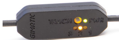
Output 2 - Gripper Mid-Stroke: (Part Gripped)
