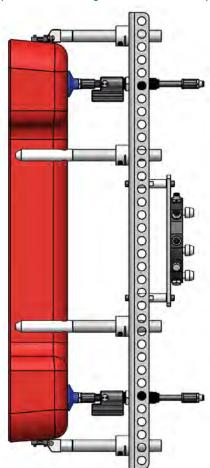
Pneumatic brake suspensions can absorb an ejection stroke and then be locked in place for degating as shown in the above application.
