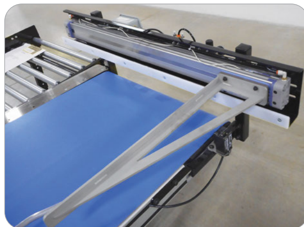
This basic sweep arm application transfers boxes from an indexing flat belt conveyor to a roller storage conveyor.
