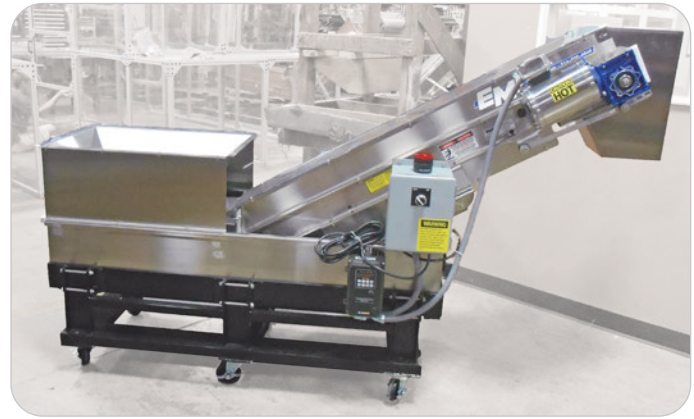
This submersible conveyor has been customized with a containment hopper and mobile floor stand for portability within the plant.
