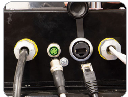
• Digital and Ethernet connections for internal and external drive.
