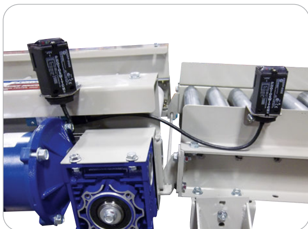
Photo eyes can be mounted to any EMI conveyor with brackets, without frame modifications.
