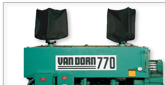
EMI clean air bags expand and contract as the machine clamp opens and closes, doing their job shot-after-shot, hour-after-hour. You can expect long, reliable life from each bag.
