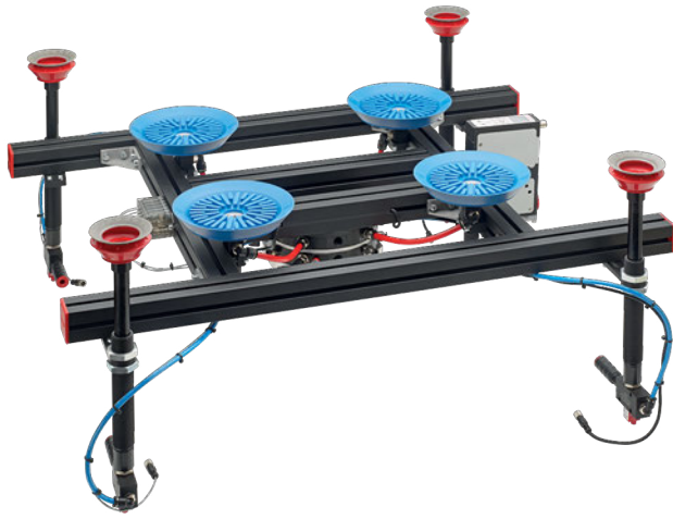
Handling of aluminium drawer units: custom solution with VG.CF mark-free suction cups in HNBR, EJ-XPRO vacuum pump with built-in control logic and decentralized pumps for feeding VG.IS suction cups for handling the protection interlayer.
