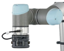
575 KIT-UR-EQC20 Electric tool changer with electric connector (kit for UR robots)
