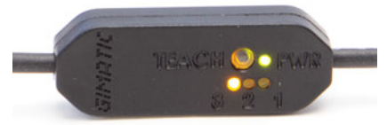
Output 3 - Gripper Closed: (Part Missed)
