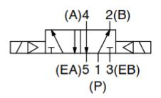
**ZONE 1 & ZONE 2** - PNEUMATIC DIAGRAM FOR GRIPPERS 5 PORT/2 POSITION, DOUBLE SOLENOID (BISTABLE) VALVE
