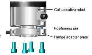
Tightly connect the ECBPMi to the flange adapter plate using the bayonet fastener. Position the ECBPMi so that the small triangle points toward the groove on the flange adapter plate.
