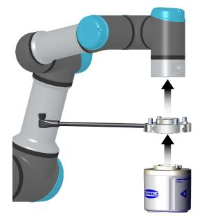
Position the flange adapter plate included in the delivery on the suitable collaborative robot using the positioning pin and fasten it using the four M6x12 cylinder head screws. Observe the permitted tightening torque for the thread.
