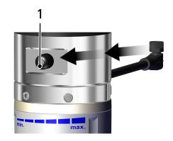
2. Optional: Use cable ties to fasten the connection cable to the drilled holes on the flange so that it is laid tightly against the robot arm.
