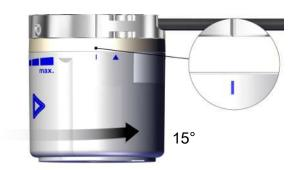
4. NOTE! End position is not reached and the line on the ECBPMi does not match the groove on the flange. Screwing in the locking screws damages the light conductors. They are then secured against being opened unintentionally with the two screws (M3x14). Observe the max. tightening torque of 0.6 Nm.
