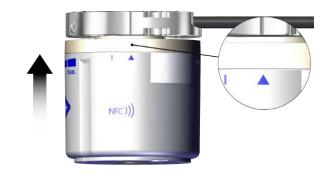
3. Turn the ECBPMi clockwise by 15° (until it stops) (the line marking matches the groove on the adapter flange).
