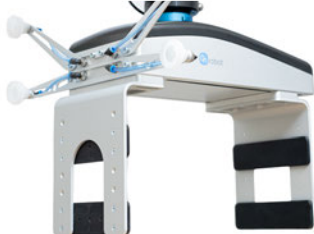
2FGP20 Palletizing Gripper with Vacuum
