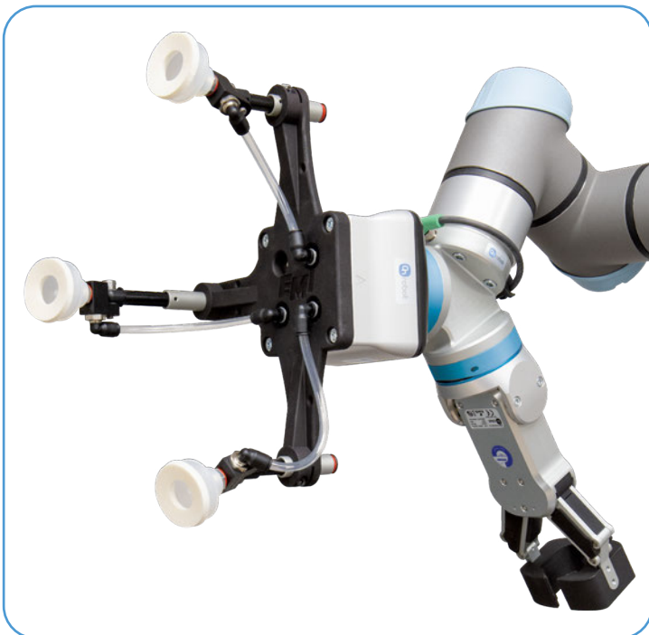
Custom 3D printed EOAT & RG2 flocked fingers
