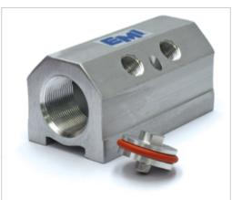
Anodized Aluminum Manifolds are available with a middle divider. The divider is stainless steel, with a silicone ring that prevents leakage. This is factory installed and field serviceable.
