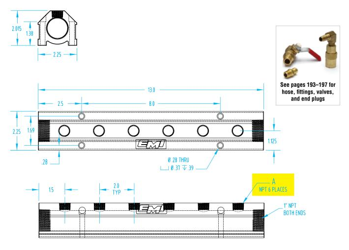
6 Outlet Aluminum Manifold with 1½" NPT End Ports Available with Middle Divider
