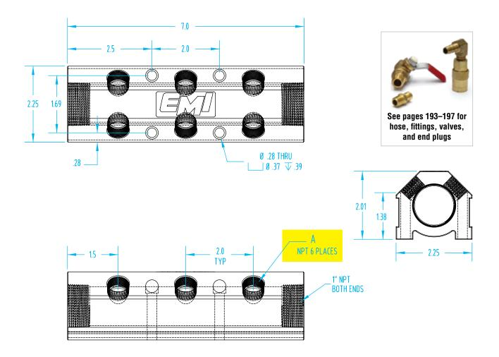
6 Outlet Aluminum Manifold with 11/2" NPT End Ports
