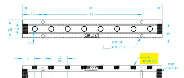
8 Outlet Aluminum Manifold with  $1^{1\!/}_{2}"$  NPT End Ports
