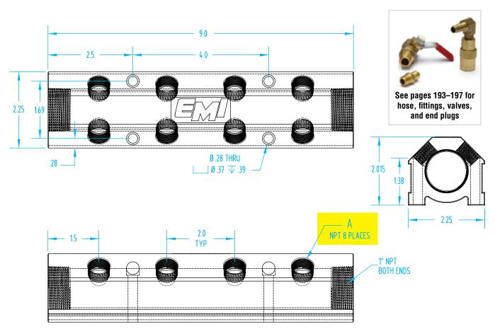
8 Outlet Aluminum Manifold with  $1^{1\!/}_{2}$  " NPT End Ports Available with Middle Divider
