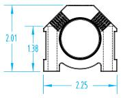
4 Outlet Aluminum Manifold with  $1^{1\!/}_{2}$  " NPT End Ports Available with Middle Divider
