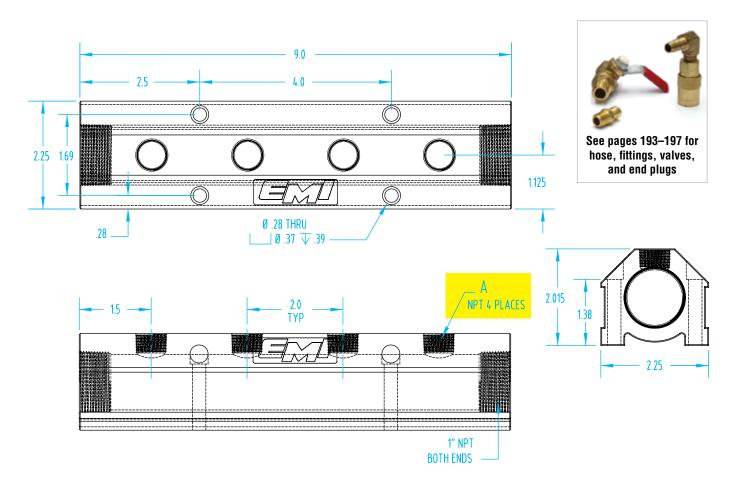
4 Outlet Aluminum Manifold with  $1^{1\!/}\!2^{"}$  NPT End Ports Available with Middle Divider
