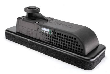
The Cobot Palletizing Tool (CPT) is a lightweight, smart and energy efficient solution intended to maximize the output of smaller robots. With a large footprint and compact gripper body design, you are able to grip multiple workpieces at once taking advantage of the piSMART valve. Available in-stock from EMI, contact our EOAT Engineering team to send workpiece samples in for testing.
