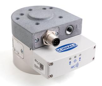
The Schmalz RECBi is a pneumatic vacuum generator that can be assembled directly on the end of a robot, or cobot. It provides powerful vacuum generation and integrated blowoff control for short cycle times and high leakage compensation. Any vacuum gripping tool, from single cups to full EOAT solutions, can be mounted directly to the end and plugged in easy application.
