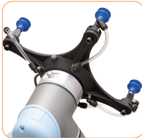
Included vacuum generator with monitoring switch for part confirmation.
