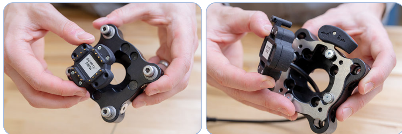
Replace the Electrical Connector back into the QC75 and fasten with the same hardware. Note that cables are meant to run down the backside grooves of the QC75 to avoid any cables from pinching.
