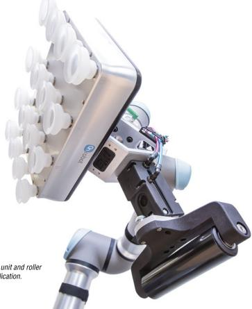
Shown with a Gimatic tilt unit and roller for a label placement application.
