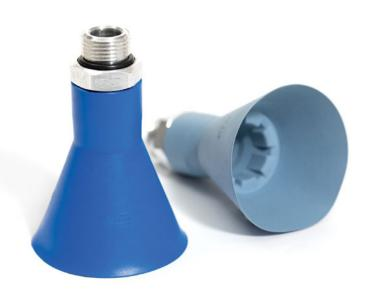
These bin-picking vacuum cups from Schmalz have an extremely thin sealing lip for optimal adaptation to corners, edges and free form surfaces. Stabilizing internal support contour for safe handling of different products. Large nominal flow compensates for leakages in a wide variety of workpieces.
