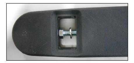
This picture illustrates the belt being tensioned by a manual setting. (Sometimes required based on belt type, machine type, machine size, etc) Bolts are turned out forcing the end cap out from the frame and thus tightening the belt.
