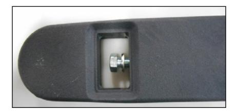
This picture illustrates the belt being tensioned by the springs. (normal / designed condition) End cap is able to "float" and maintain belt tension.
