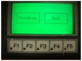
Program Pushbutton: Goes to Program screen Run Pushbutton: Goes to Run screen
