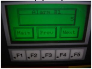
Alarm #1 Pushbutton: Goes to Numeric entry screen
