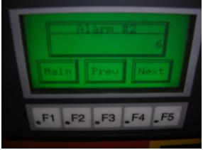
Alarm #2 Pushbutton: Goes to Numeric entry screen
