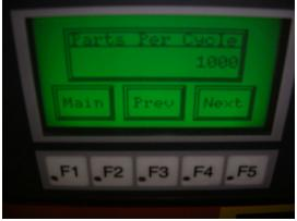
Parts per Cycle Pushbutton: Goes to Numeric entry screen
