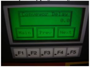
Conveyor delay Pushbutton: Goes to Numeric entry screen
