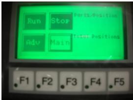
Run Pushbutton: Starts system cycle
