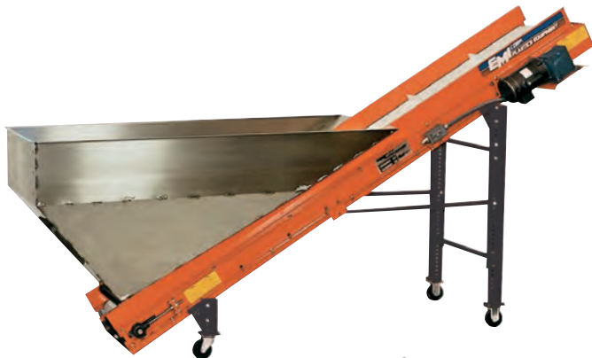
A Model RMC-18-10-20 conveyor (set at a 30° angle) with optional castors and a 20 cubic foot capacity stainless steel infeed hopper.
