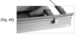
After both extension rails are mounted, bolt the back end rail in place using 1/4" bolts supplied. Make sure both the end rail and the end rail flapper line up with each other. The belting on the end rail should come down over the end flapper to close up any gap. (Fig. 44)
