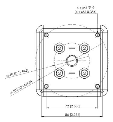
The Push-in Fittings are used to attach 4 mm vacuum tubes to create customized configuration that required remote vacuum. In most cases, this size is enough for generating the needed vacuum from the pump in the gripper.
